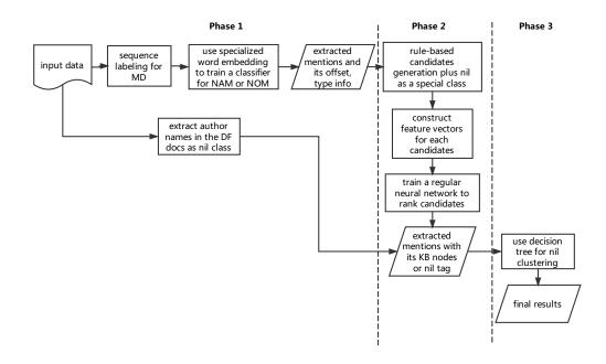
Figure 1: The flow chart of EDL system
